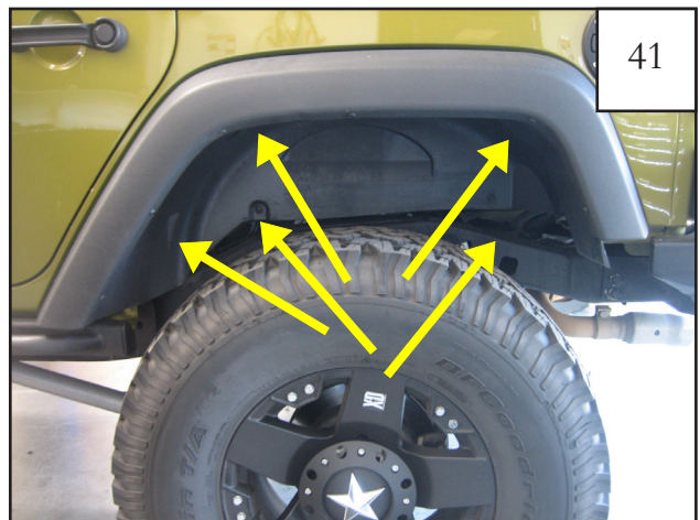
Using a pry tool, pliers, or flat head Boltdriver, remove four plastic fasteners from inside of splash shield.
