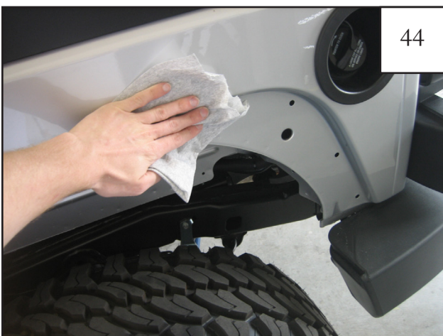
Thoroughly clean the exposed metal fender with a damp cloth then dry, and apply masking tape to protect painted surface.
