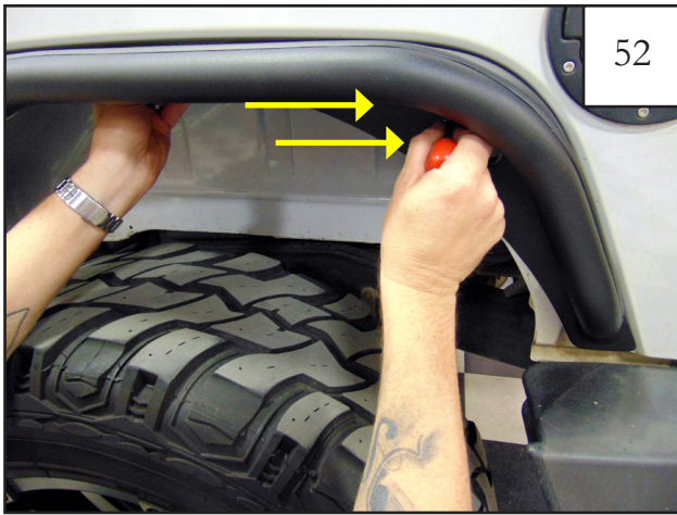
Test fit rear flare and use a grease pencil or awl to mark (2) hole locations in preparation for drilling.
