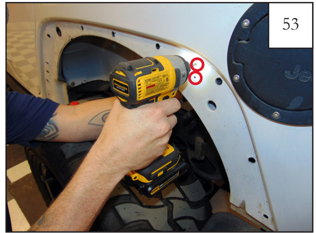
Drill (2) pilot holes using 1/8" drill bit, and finish with a 3/8" drill bit.
