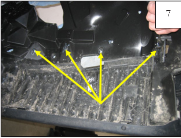
Use a pry tool or flat head Boltdriver to remove four plastic fasteners.
