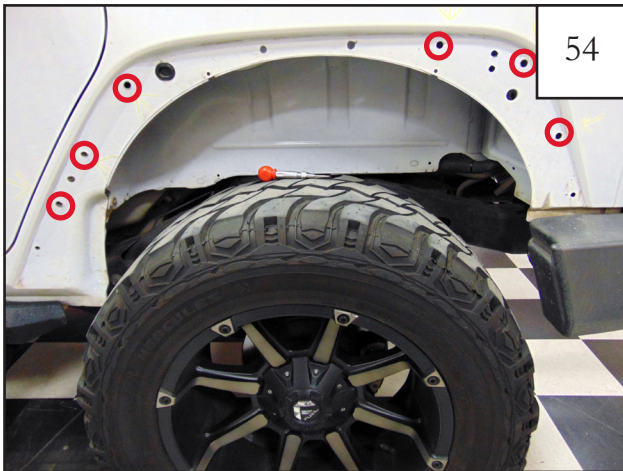
Drill out (6) factory hole locations shown above using 7/16" drill bit, in preparation for installing rivnuts.
