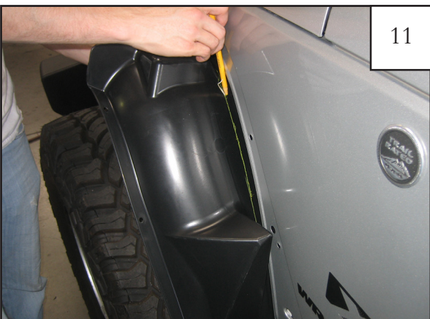
Using sheet metal as a guide, mark the rear portion of the splash shield with a grease pencil. The splash shield should be flush with the sheet metal after being trimmed. NOTE: If trimmed too little, flare won't fit; if trimmed to much, shield won't stay behind flare.
