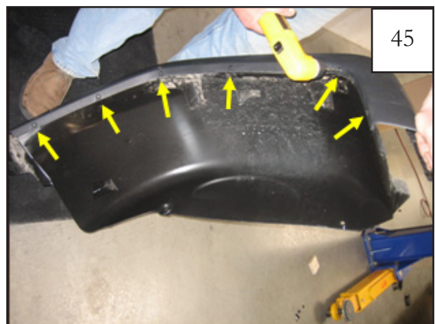
OPTIONAL: If reinstalling inner fender liner, follow Steps 45-51 . Use a drill with a 5/16" bit to drill through six plastic rivets along edge of flare/splash shield. Discard the flare. Save splash shield for reinstallation.
