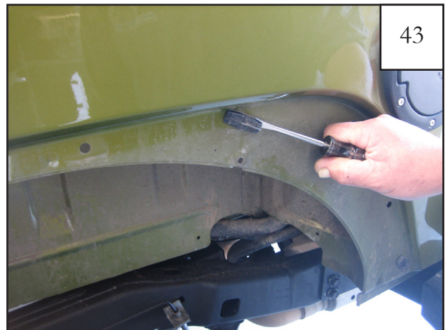
Using a pry tool or flat head Boltdriver, remove any plastic clips still in fender.
