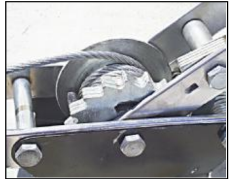
Figure 2 Close-up of the ratchet mechanism lock tooth wheel
