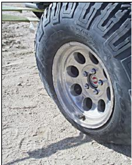
Figure 16 The deflated, winched tire was pulled until it began to drag sideways. Still no bead pop.
