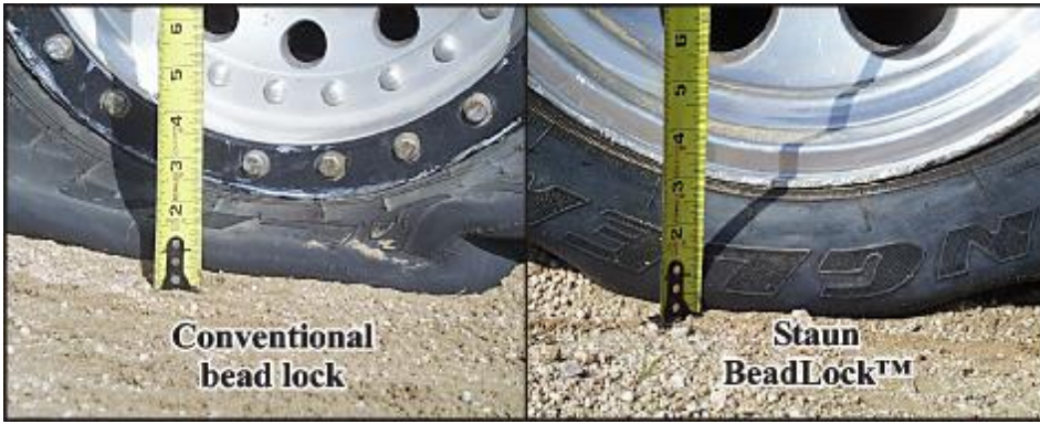
Figure 4 The conventionally bead locked tire on the left has to endure more stress than the Staun BeadLocked tire on the right when flat. The Staun-protected tire and rim are raised by the internal tube thus reducing stress.
