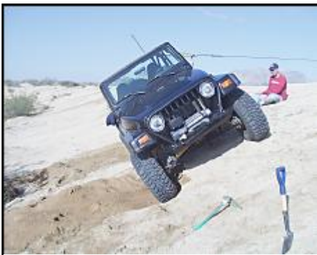
Figure 13 With maximum side tilt achieved, note that the highside tires look a little "light."
