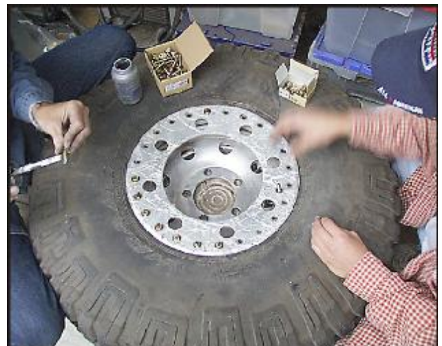
Figure 3 In a blur, the conventional bead lock ring and 24 cap screws became one with the wheel.
