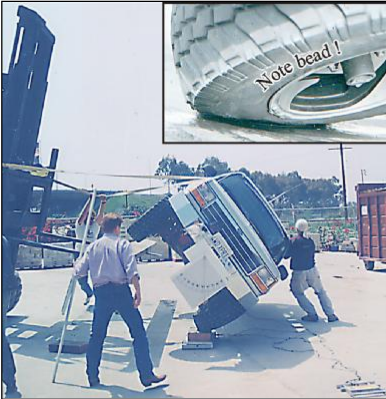
Figure 2 Demonstrating properly inflated bead, load capacity. Upper right shows tire sidewall distortion. Vehicle is pretty much in balance. We lifted the highside wheels with a board (shadow obvious) to simulate ground with Norm Clow (out of sight) driving his "Big Bertha" fork lift, and me "balancing" with my shoulder. Note safety tethers (top of 4X) and Rancho-furnished strain gauges under lowside wheels. Carefully study the angle of the rim independent of the tire. This reveals a lesser angle than first apparent. I surmise that the apparently "okay" sidewall is significantly "sideshifted" by ground contact. That's with the vehicle balanced at about 50+°.
