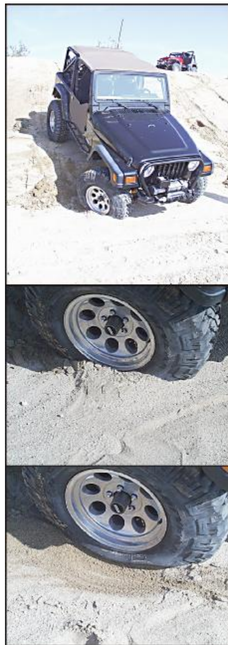
Figure 15 To create more severe, instant, bead breaking force, we drove Brian's TJ off a three-foot bank (top) at an angle, forcing the right front tire into the ground (center). Exposed buried tire shows additional weight transfer stress (bottom), but no air or bead loss.
