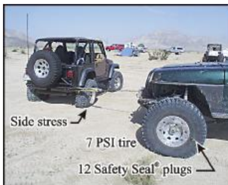
Figure 11 Note: 1) side stress on deflated tires; 2) 7 PSI tire for reference and 3) Safety Seal® effectiveness.
