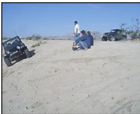
Figure 10 Side tilt test setup prior to making steeper. Master-Pull safety tether to TJ on right almost invisible.
