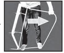
Step 3. To adjust the door frame towards the windshield you will need to adjust in the opposite direction as illustrated using the same procedures as in step two.
