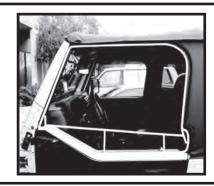
Step 2. To adjust the door frame properly you will need a flat even surface. To adjust the door frame away from the windshield you will need to stand the frame vertical on the ground with the windshield side on the ground. Stand on the lower portion of the frame and using slight force adjust the frame in the direction illustrated. Adjust the frame in small increments and test fit after each adjustment until the desired fit is achieved.
