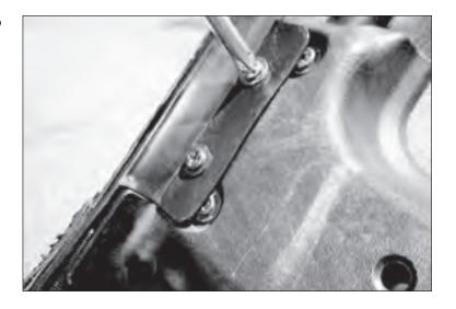
6. Raise top and bow assembly in upright position and lock header to windshield. Carefully drape soft top fabric over windshield and remove all screws from top side of header. Remove top of header and soft top fabric.
