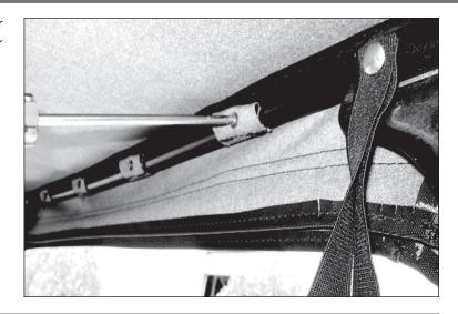
4. Unfasten hook and loop retainer that secures top to bow above roll bar and lower soft top.
