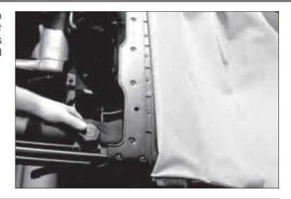
7. Place new soft top fabric on header with bottom side facing upward. With fabric draped over windshield, locate and align center notch on fabric and header. If necessary, use tape to hold fabric in place. Reattach top portion of header using screws removed in step 6.
