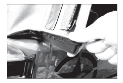
12. Insert tailgate bar into new rear window and install rear and side windows. Secure top above doors by inserting plastic retainer strips in door surrounds.
