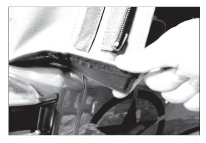
3. Remove both sets of phillips head screws on rear bow and set aside for later use. DO NOT use power tools.
