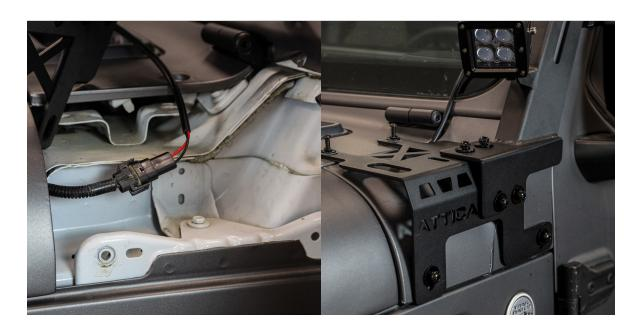
Wire up the power and ground based on your switch setup. And attach the bracket to the vehicle using **W09**, **W13**, **W14**, **W16**, **W17**, and **W19** washers, **B10** and **B23** bolts.
