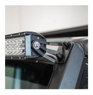
Next step will be to mount the light bracket using **N12** nuts, **B15** bolts and **W09** washers.
