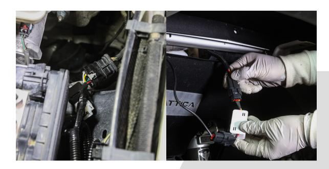
Locate the OEM turn signal harness from the top right of the engine room and connect it to the Attica Terra Series Front Fender Flare light using the adapters.
