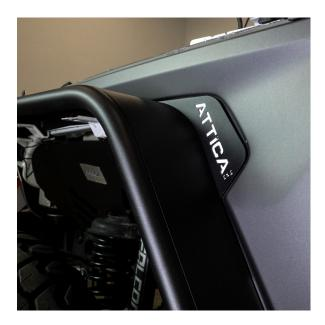
Start by installing our Jeep Terra Series Fender Flare onto the vehicle, including the plate, using N14 nuts, W23 washers, and B15 bolts.
