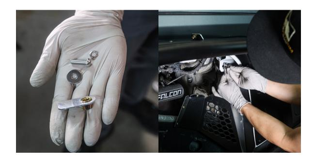
Secure the top mounting point using the threaded plate, **B61** bolts, **W38** washers, and **W08** washers. Use a **4mm hex tool** for this step. For the remaining mounting points, use **N30** nuts.
