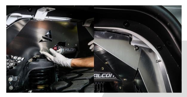
The next step is to install the larger inner fender liner. Position the liner as shown in the images above.
