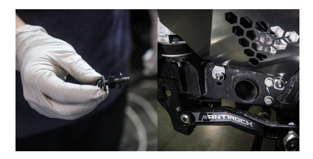
The lower two mounting points require **R01** rivet nuts, **W41** washers, and **B62** bolts. Secure them using a **5mm hex tool**.
