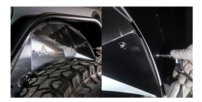
Using **B61** bolts, **W08** and **W38** washers, and **N30** nuts, mount the liner to the body using a **4mm hex tool**. Next, attempt to tighten all the inner fender bolts that were previously hand tight.
