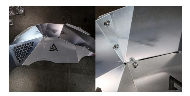
Preassemble the rear inner fender liner using **B60** bolts, **W08** and **W38** washers, and **N30** nuts. Leave the bolts finger tight, as they will be tightened in a later step.
