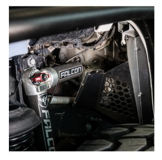
Start by installing the smaller part of the inner fender onto the vehicle.
