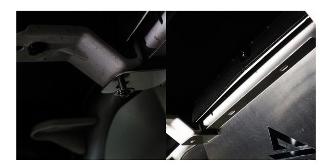
The top mounting points require **B61** bolts, **W08** and **W38** washers, and **N30** nuts. Secure them using a **4mm hex tool** and a **10mm wrench**.
