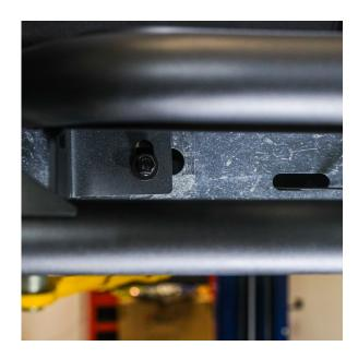
The front mount is fastened with **B35** bolts and secured in place using **W22** and **W23** washers. These components are connected to the threaded plate using a **12mm** and **16mm socket tool**.
