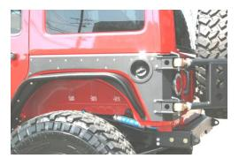
48. Coilover Reservoir tabs can either be mounted on the outside of the frame or on the EVO subframe with Bypass Reservoirs. Use two tabs and two hose clamps per reservoir.
