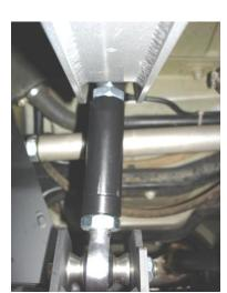
39. Using ½" hardware install opposite end of EVO endlink into passenger side axle mount
