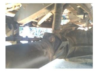
40. Assemble EVO cross brace links, thread jamb nuts on each heim and thread each heim into cross brace tube.
