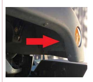
Using the 10mm socket and flat head screw driver, remove the bolts and clips for the inner fender liner. Remove the inner fender liner. If you have the JcrOffroad Front Inner Fender Kit, you can dispose of the stock liner. If you did not purchase the JcrOffroad Front Inner Fender Kit, then place the stock liner to the side for later installation.
