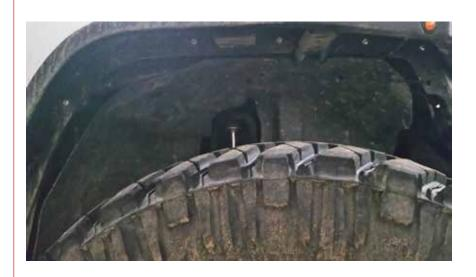
The side marker holes in the fender flares are made to accept any 3/4 mini auxiliary LED lights.
