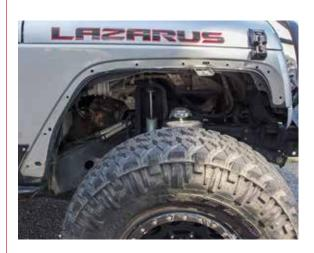
If you did not purchase the JcrOffroad Front Inner Fender Kit, now you will need to mark and trim your stock inner fender liners. Using the front and rear mounting bolts, reinstall the liners. Using a marker, mark where the liner sticks out from the body. Remove the liners and cut them where you have marked using a utility knife.
