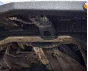
**9** Now thread all the rest of the bolts and nuts loosely into place. Make final adjustments for placement of the fender, then tighten down all the hardware.
