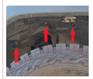
3 Using the 1/4 drill bit, drill and flat head screwdriver, remove the clips and bolts holding the fender in place. Then drill out the plastic rivets along the outside edge that are holding the fender to the inner supports. Remove the stock fender.
