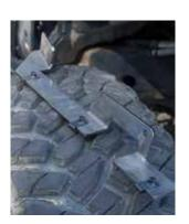
**C** Reusing the stock bolts and a 10mm socket, install the upper support bracket through the two holes on the bottom of the bracket.
