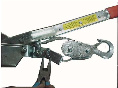
2. Pull the pin and separate the cable from the hoist mechanism.
