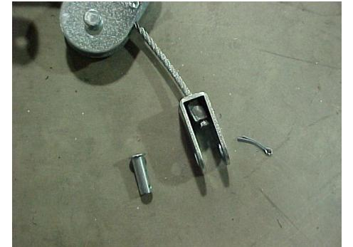
3. Insert the eyebolt as shown. Rein-stall the cotter key and bend one arm of the key to prevent separation of components. Check all connections.
