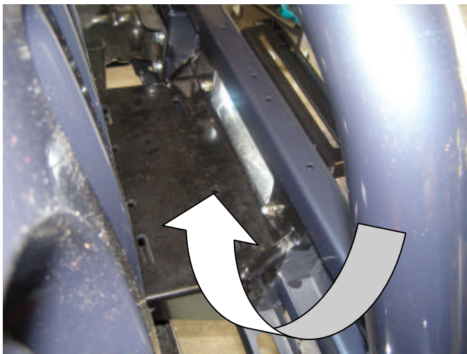
WINCH MOUNTING PLATFORM
