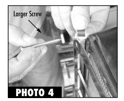
Now using the new screws (provided), insert the larger screw (#8) through the outside top hole and through the spacer (provided). Insert the smaller screw (#6) through the inside top hole and through the spacer.
