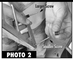
Using the new screws (provided), insert the larger screw (#8) through the outside bottom hole and the smaller screw (#6) through the inside bottom hole. Then place the spacers (provided) on each screw.
