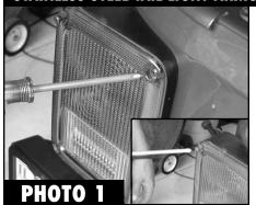
Begin by removing all four screws from the tail light. You will **not** use these screws for installation.
