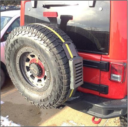
After Installing bracket, ensure that the bracket does not interfere with vehicle functionality.
