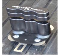
Please the mount onto the side panel of the bed rack. The position will be determined how many tanks you want to mount on your bed rack
