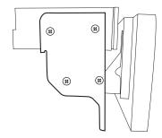
6 Route the key harness through the top-left side of the i209 source unit. Mount the i209 source unit using (4) 7mm factory screws.
