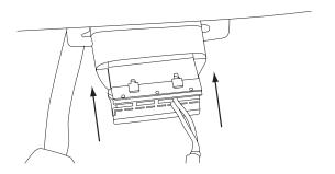
2 Remove the vents from the radio section on the OEM dash panel by pressing down on the lock tab and turning right. Mount vents on to the i209-WRA bezel.
