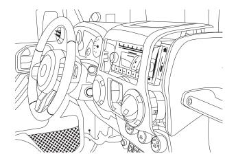
6 Extract (2) 7 mm screws from the factory radio bracket and remove it.
