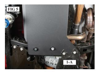
Torque M10 bolts to 36 ftlbs and M12 bolts to 48 ftlbs.
