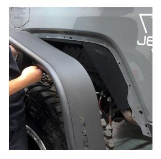
The mounting points require **B15** bolts, **N14** nuts and **W19** washers. Secure them using a **4mm hex tool**.
