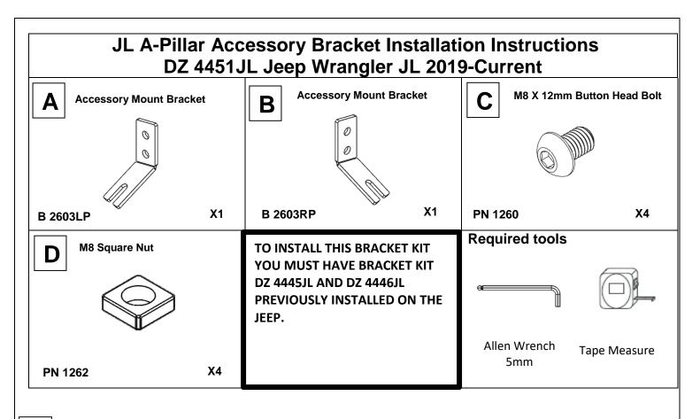
Install bolt (C) through the bracket (A) and put a nut (D) on the back side and slide the bracket in the channel and locate the desired position. Fully tighten bracket.
