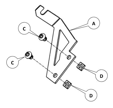
Slide bracket into A-Pillar channel and replace endcap. Fully tighten endcap at this time.
