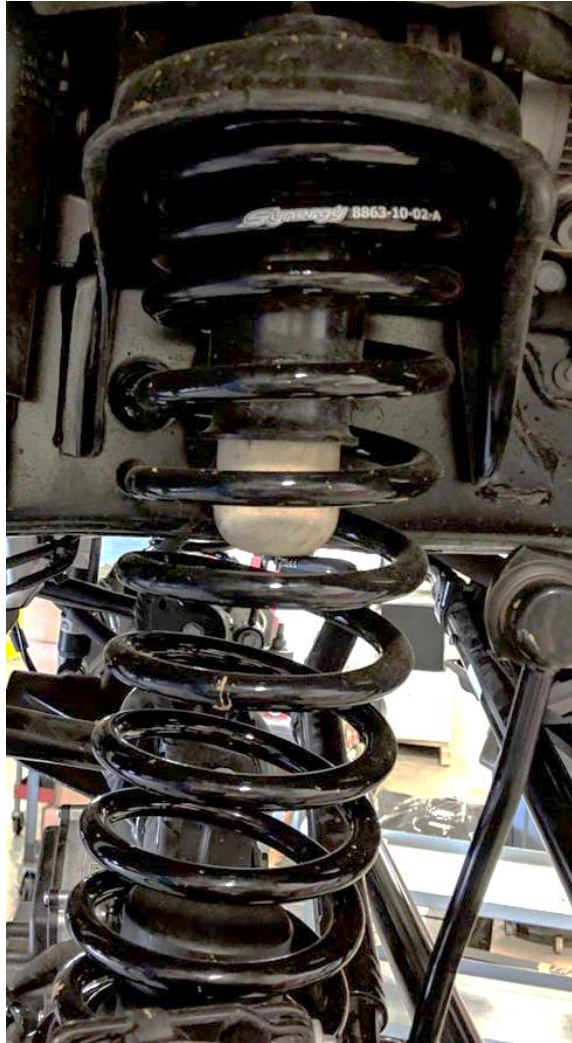
Figure 2. Correctly Installed Front Coil Spring
