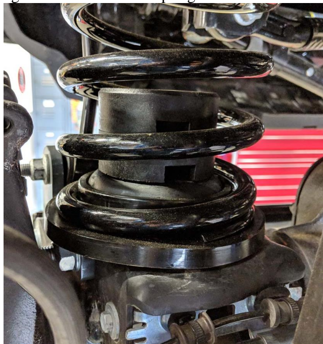
Figure 1. Correctly Installed Lower Spring Isolator
