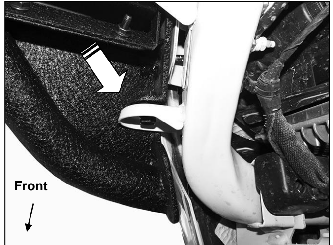
(Fig 9) Attach front of Fender to mounting tab on body (arrow)
