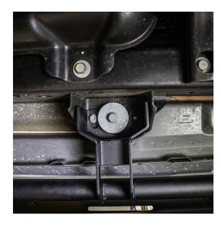
The middle mount uses **W23** washers and **N17** nuts with a **15mm socket tool**.
