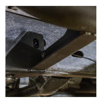
The front mount is fastened with **B35** bolts, **W22** and **W23** washers. These components are connected to the threaded plate using a **16mm socket tool**.
