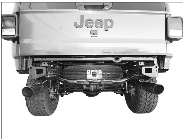
(Fig 7) Factory bumper removed
