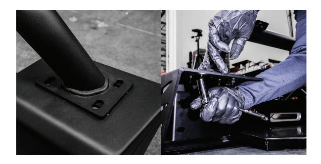
Align the mounting points of your bull bar with the top of your front bumper as shown above. It mounts to the front bumper using your **B19** bolts, **W19** washers and **N14** nuts with **5mm hex tool** & **13mm socket tool**.
