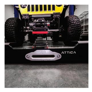
Start by installing the winch guard into place on the main center section of the bumper.
