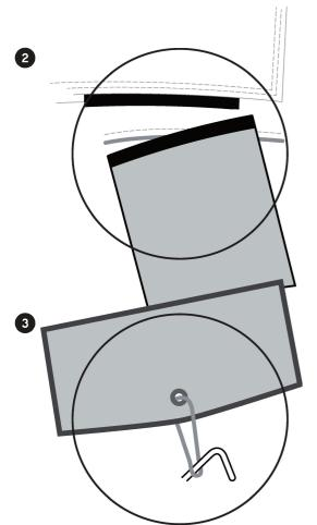
Connect the wall to the awning by using the zippers. Align the starting point of the shade wall zipper to the starting point of the awning zipper. Once aligned, pull the zipper to the other end of the zipper tract. 2 people make this process easier.
