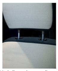
Finish installation by adjusting the seat covers around and behind all seat levers, adjusters, covers, and trim. Seat covers can be carefully tucked under and around the headrest grommets. This will provide a more finished look and retain access to headrest release tabs. (Fig 3) Finally, install headrest covers and reinstall headrests. (Fig 4)
