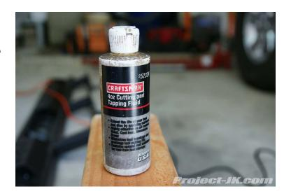
16. With the help of some cutting oil, slowly and carefully tap all your mounting holes. Due to the body of the Jeep JK Wrangler being in the way, you will not be able to use a standard tap handle to do this. I improvised and used a wrench to do this job.
