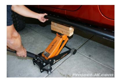
7. Using the factory hardware, secure your new LoD Signature Series Rock Slider to the points where the automatic transmisson and transfer case skid plates attach the frame rail on your Jeep JK Wrangler. An 18mm socket will be needed for this job.
