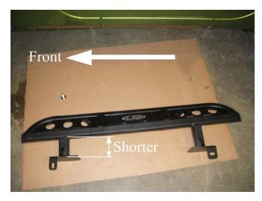
**6.** Place your LoD Signature Series Rock Slider on a floor jack and carefully maneuver in place under your Jeep JK Wrangler's driver side rocker panel.
