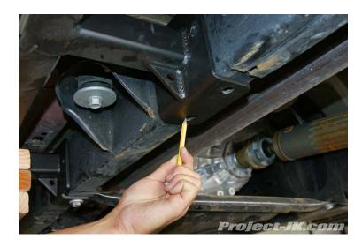
**10.** Remove the 2 bolts securing your LoD Signature Series Rock Slider onto the frame rail and then carefully lower and remove it from your Jeep JK Wrangler.
