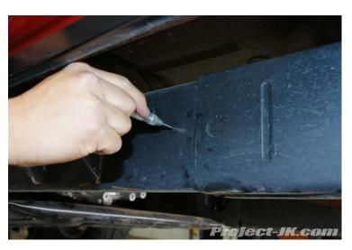
**12.** Using a small metal drilling bit or Unibit, begin drilling pilot holes on all the mounting points on you've marked off your Jeep JK Wrangler's frame rail.
