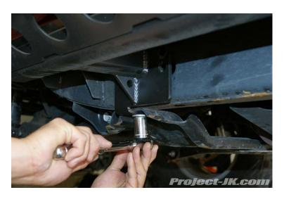
19. Using the 7/16"x1" bolts that come with the kit, secure your LoD Signature Series Rock Slider onto the new mouting holes that you made on your Jeep JK Wrangler's frame rails
