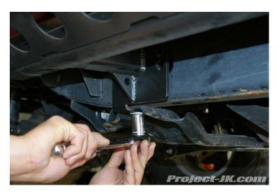
8. Double check that your LoD Signature Series Rock Slider is sitting straight. Then, using it as a template, mark off all the mounting holes you will need to drill out on the side of your Jeep JK Wrangler's frame rail.
