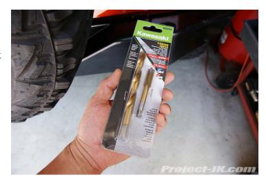
**14.** Using the drill bit that comes with the drill and tap set, finish drilling out all the pilot holes that you made back on step #11.
