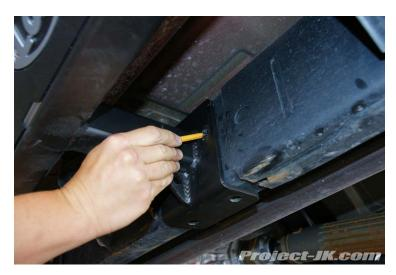
**9.** On the mount closest to the rear tire, there are 2 holes on the bottom of your Jeep JK Wrangler's frame rail that you will need to mark off as well.
