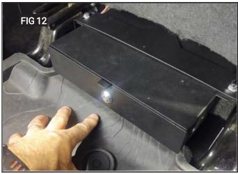
After installation confirm proper seat function. Seat should slider fully forward and fully back without interference. Confirm proper key and drawer operation (Fig11). Reinstall floor mat or floor liner (Fig12).
