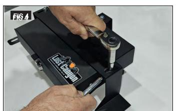
Flip assembly over and center Security Box in Mounting Bracket slotted mounting holes (Fig3). Using M10 wrench, M10 socket and ratchet secure Under Seat Security Box to Mounting Bracket using supplied M6 Nylock nut, washers and bolt. (Fig4).
