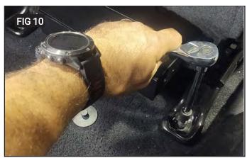
Place Security Box Mounting Bracket under seat mounting bracket. Align seat mounting bracket holes with Security Box Mounting Bracket holes and reinstall factory T50 Torx bolts removed in step 4 (Fig9). Using T50 Torx socket tighten seat mounting bolts and torque to 45ftlbs (Fig10).
