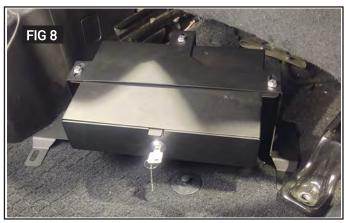
Using T50 Torx socket loosen and remove the two rear seat mounting bolts securing seat base to floor. Do Not Discard T50 Torx bolts. They will be reinstalled in step 5 (Fig7). With bolts removed lift back of seat up and slide Under Seat Security Box assembly under seat brackets (Fig8).
