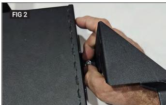
**Put on safety glasses.** Place Mounting Bracket upside down onto a flat surface. Insert M6 Hex Head Bolt and Flat Washer through mounting holes (Fig1). Flip Under Seat Security Box over and align mounting tabs with corresponding holes on Mounting Bracket. Attach M6 Flat Washer and M6 Nylock Nut to M6 Hex Head Bolts (Fig2)
