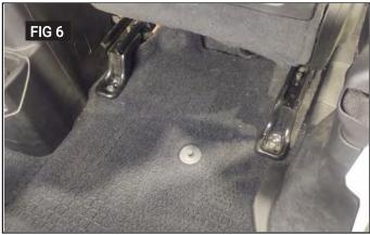
Slide front passenger seat fully forward. Remove any loose articles from around and under back side of passenger seat (Fig5). Remove floor mat or floor liner. To be reinstalled later (Fig6).
