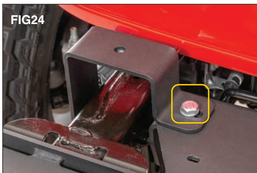
Loosely install the OEM hardware removed in FIG 20 inside the frame rails using spacer plates (if necessary) to center winch mount best as possible. (FIG 22)
