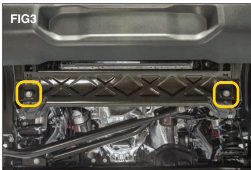
Remove the two bolts holding on the Original Equipment cross shield using a 16mm socket. Remove the cross shield by lifting upward and out. Note: This will not be reused with your new bumper. (FIG3)
