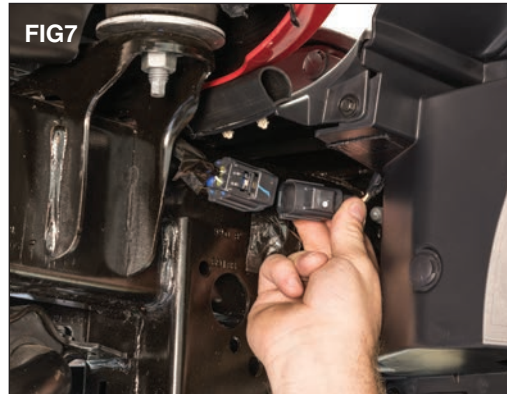
Lastly disconnect the fog light wiring harness plug so the bumper can be removed. (FIG7) Carefully remove the bumper from the frame rails.
