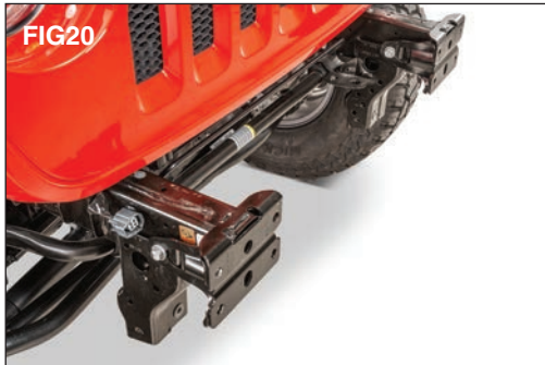
Remove the 4 bumper support brackets using a 16mm socket and set hardware aside for re-use later. (FIG 20)
