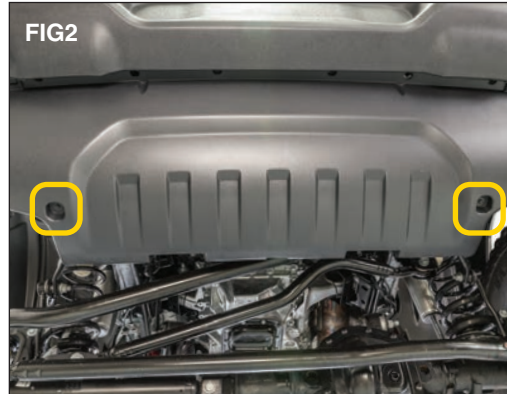
Remove the two screws on the underside using a 5/16" socket. (FIG2) Remove the splash guard. Note: This will not be reused with your new bumper.
