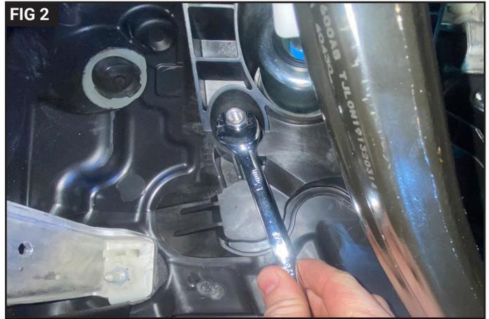
Put on Gloves and Safety Glasses. Locate the lower left Brake Booster firewall bolt. (FIG 1) Thread the M8 Coupler on to this stud and tighten with a 13mm box end wrench. (FIG 2)
