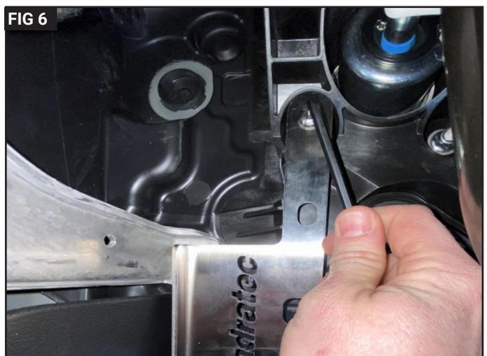
Align the Dead Pedal Mounting Bracket with the previously installed Coupler. (FIG 5) Thread the M8 Socket Head Cap Screw through the bracket and into the coupler on the firewall. Tighten with a 5mm Head Key. (FIG 6) When installation is complete, be certain to verify that any floor mat or floor liner you are using does NOT interfere with your throttle or brake pedals in any way.
