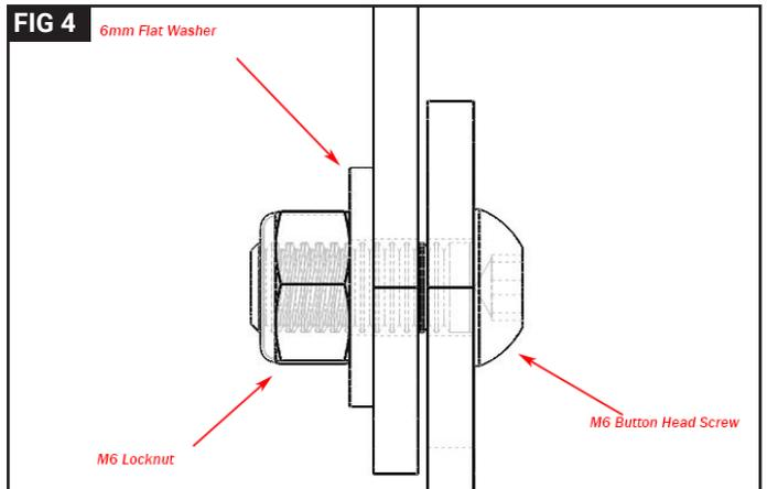
Next, assemble the pedal to the mounting bracket as shown. There are 3 possible different positions for height/angle options. With the M6 hardware, assemble the pedal and bracket to your desired angle/location using a 4mm hex key and 10mm open end wrench. (FIG 3 & 4)
