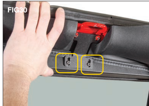
While pushing up on the light bar as much as possible tighten the torx screws into the light bar. (FIG 30)
