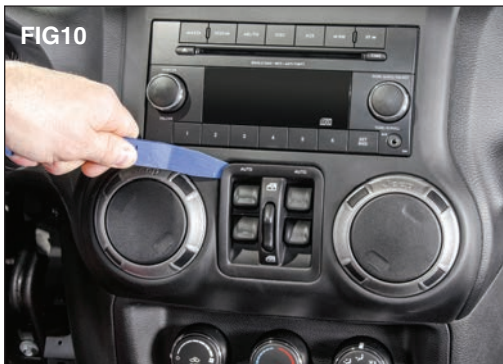
Using a trim clip removal tool gently remove the window control switch or dash pocket if switches aren't present. (FIG 10)
