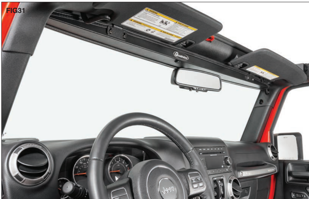
Installation is now complete.
