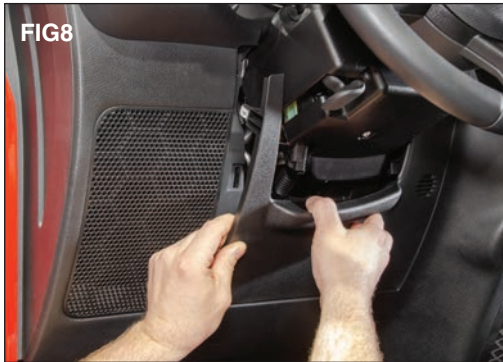
Under the steering column remove the center panel by pulling it away from the dash releasing the clips. (FIG8)
