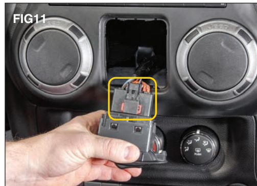
On the window control switch slide the red locking tab over, squeeze the black tab and disconnect the harness. (FIG 11)
